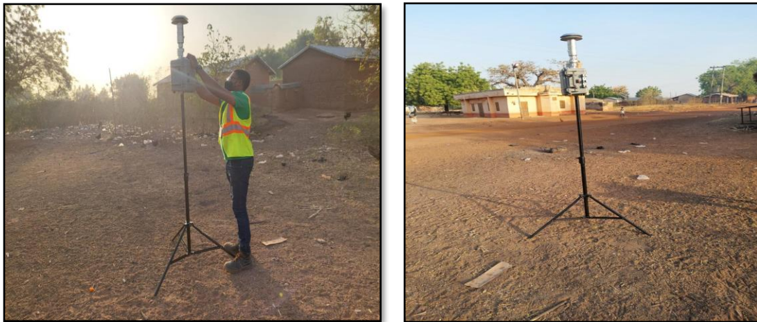
Plate 1: Setting up ARA N-FRM sampler for Ambient Air Quality Monitoring
