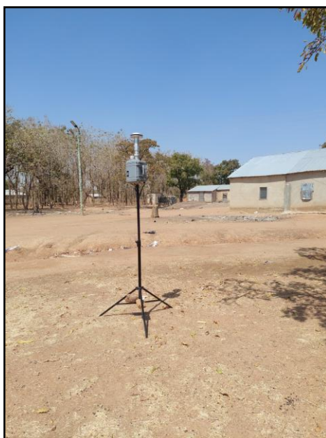
Plate 1: ARA N-FRM sampler mounted for Ambient Air Quality Monitoring
