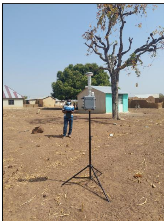
Plate 1: ARA N-FRM sampler for Ambient Air Quality Monitoring
