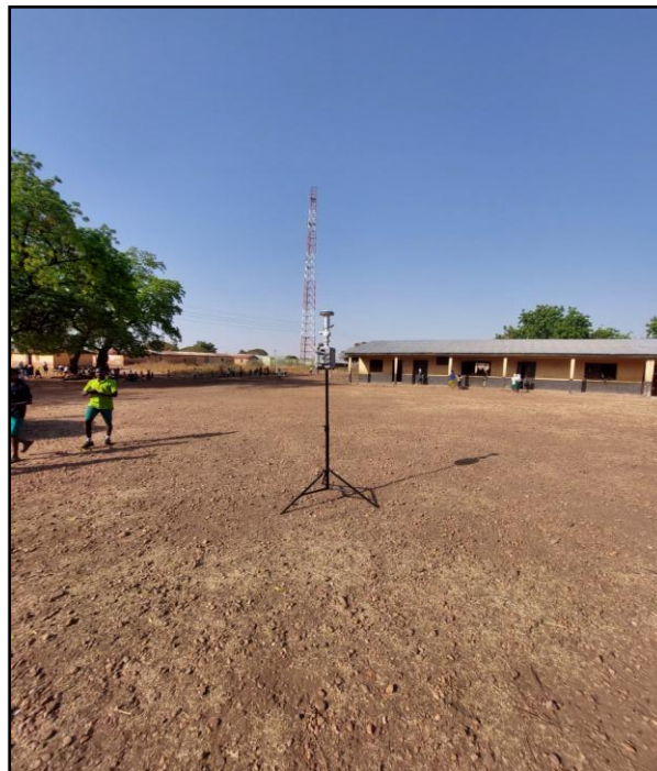
Plate 1: ARA N-FRM sampler set up for Ambient Air Quality Monitoring
