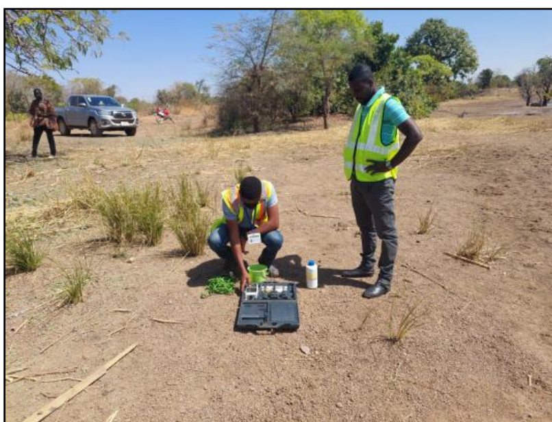
Plate 5 Ko Dugout sampling and in-situ testing.
